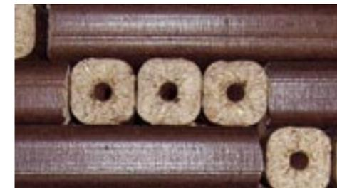
processes. The sawdust is compressed and the lignin contained in the wood can be softened, allowing it to act as a natural binder, producing a reformed log size product. Briquettes are dense and this reduces the amount of storage space required. They are clean to handle and easy to take home in 'ready to burn' retail packs.
